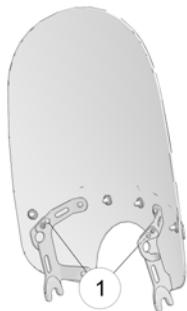
2. From the front of the motorcycle, pull firmly on the upper windshield to remove the windshield from the upper mounts, then pull the windshield upward and away from motorcycle.
