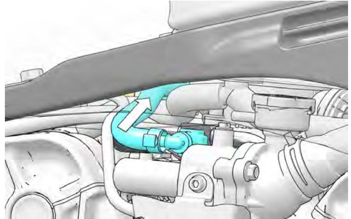
10. Lift the rear of the fuel tank and slide rearward to release from the front isolators.
