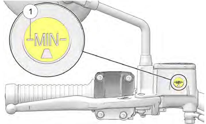
3. The fluid level should be above the minimum indicator mark in the sight glass.
