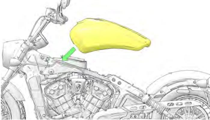
4. While supporting rear of fuel tank, connect fuel line to pump.
