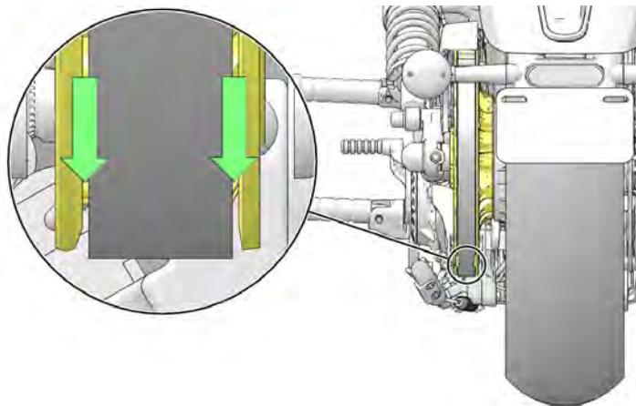
2. Rotate wheel **FORWARD** and verify sprocket teeth are still visible on both side of drive belt.
