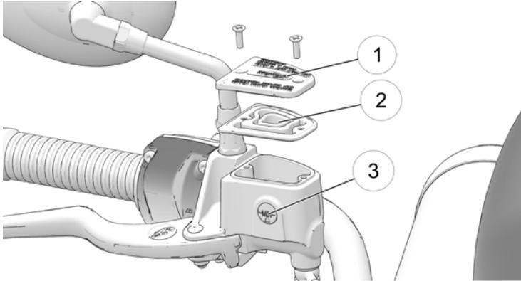
4. The fluid level should be above the minimum indicator mark in the sight glass ③. Add brake fluid as needed. *Do not overfill.*
