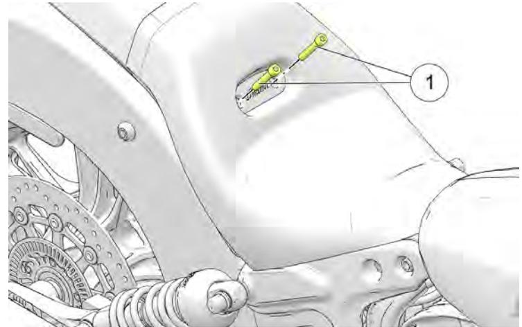
1. Remove the bolts on the back of the seat ① using the included uni-tool.
