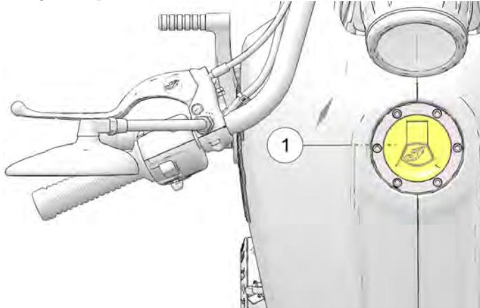
4. Add fuel to the tank until it crests the oval-shaped opening ② in the filler neck. The tank is full at this level. Do not overfill the fuel tank.
