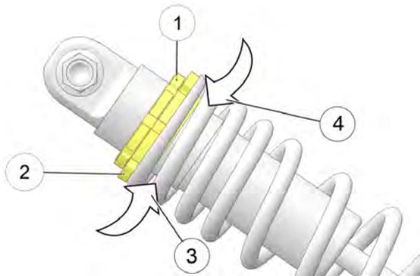
4. Spray a light lubricant on the adjuster nut where it contacts the spring. DO NOT allow spray to contact the drive belt.
