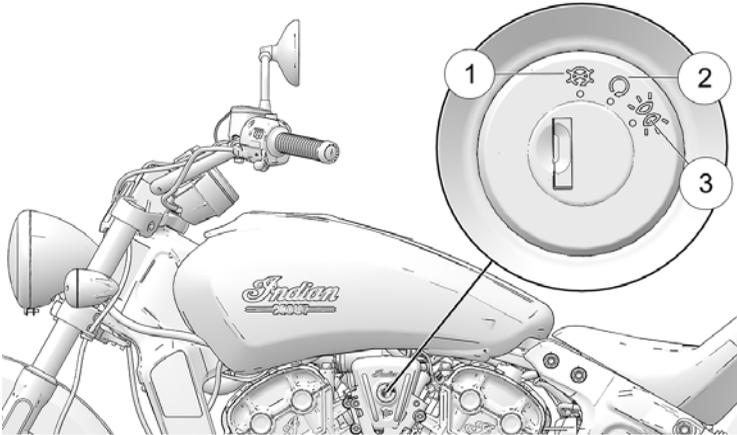
Turn the ignition switch to the OFF position and remove the ignition key when leaving the motorcycle unattended.
