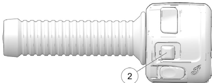
To activate the hazard switch, press on the center of the turn signal switch ②.
