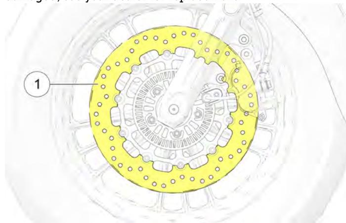
2. Clean discs if minor squeaks develop due to dirt or dust. Apply brake cleaner to a clean shop towel and wipe the discs. DO NOT allow brake cleaner to contact painted or plastic parts. Read all precautions on the label.
