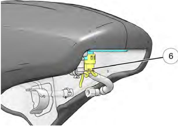
9. Gently feed fuel rail end of the fuel hose toward the center of the vehicle. Ensure the hose and connector are clear of coolant hose and all wire harnesses.
