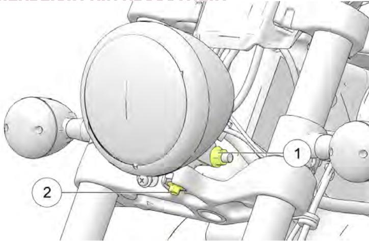
1. To adjust the headlamp vertically, loosen the housing mount fastener ① and pivot the housing upward or downward. Tighten the fastener.
