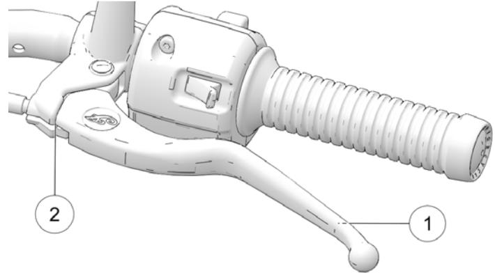
2. Freeplay (gap) is the amount of lever movement from the rest position to the point of cable resistance. Clutch lever freeplay should be 0.5-1.5 mm. Measure the gap between the clutch lever and the lever housing
