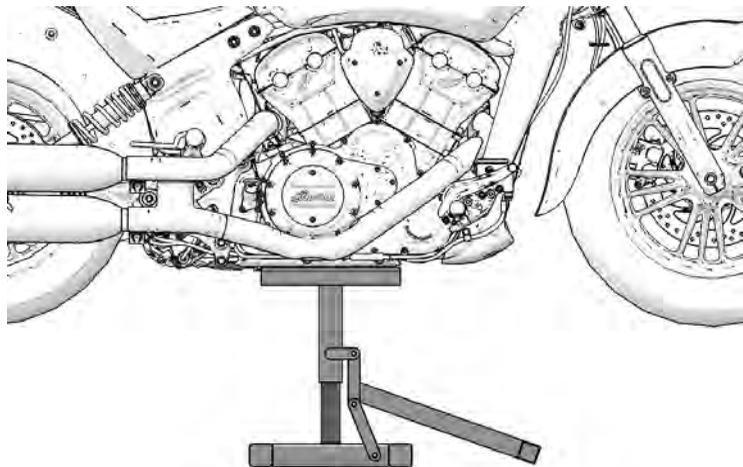
Position motorcycle platform jack beneath engine case, avoiding oil drain plug, and lift motorcycle so front wheel is off ground. Stabilize motorcycle in upright position with tie-down straps (or equivalent). Motorcycle **MUST** be stable prior to performing belt maintenance procedures.
