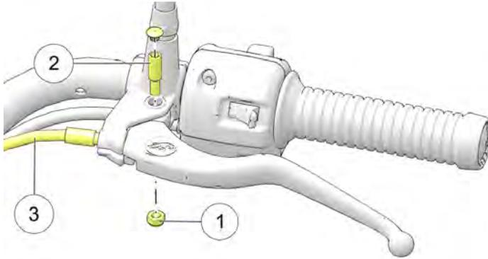
2. Remove any old grease and dirt from the lever and housing. Lubricate the clutch lever and pivot screw with moly assembly grease or all-purpose grease.
