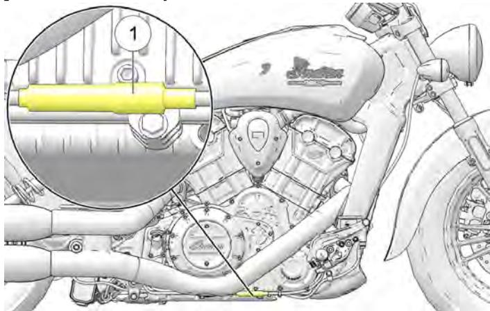
2. While holding the cable, turn the cable adjuster inward or outward until clutch lever freeplay is 0.02–0.059 in (0.5–1.5 mm) ②.
