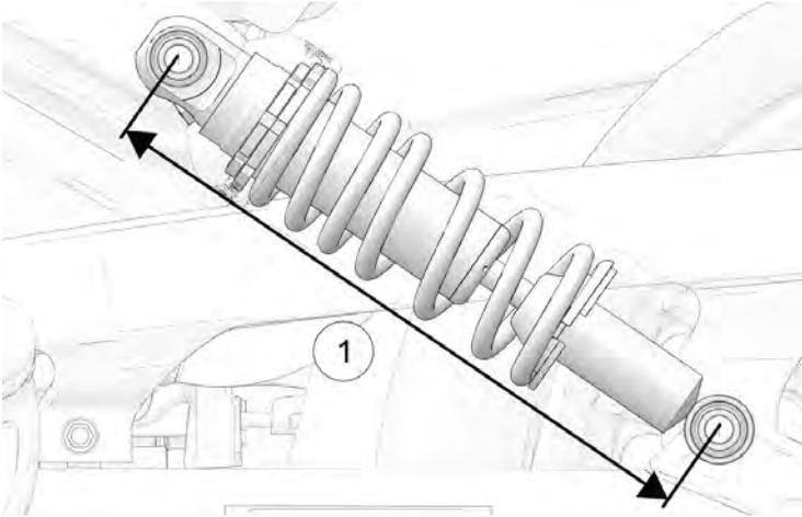
3. Measure shock preload from upper mount bolt center to lower mount bolt center (eye-to-eye) ①. Perform this measurement on both shocks.
