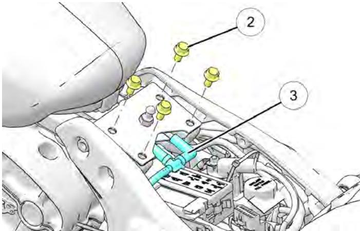
8. Connect the fuel tank vent line and the fuel cap recess drain line ③.
