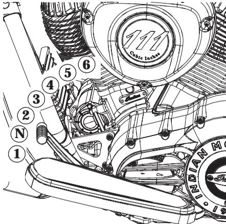
Press downward on the toe lever to shift to a lower gear. Lift upward on the toe lever to shift to a higher gear. Release the clutch lever after each gear shift.
