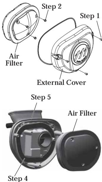
7. Reinstall the three screws. Torque to specification.
