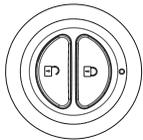
6. Press and hold the starter switch to engage the one-touch starting feature, which activates the electrical system and starts the engine. Another option is to turn the power switch on, and with the throttle closed, press and release the starter switch to start the engine. The starter motor will crank until the engine starts, but no more than 3 seconds. If the engine does not start, wait five seconds, then try again.
