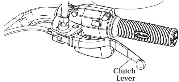
2. Freeplay (gap) is the amount of lever movement from the rest position to the point of cable resistance. Clutch lever freeplay should be 0.5-1.5 mm. Measure the gap between the clutch lever and the lever housing. See page 95. Adjust clutch lever freeplay if necessary.
