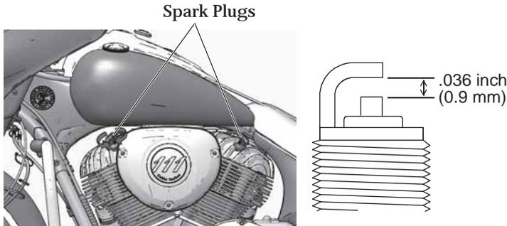
4. To prevent debris from entering the spark plug holes, use compressed air to clean the area around the plugs before removing them.
