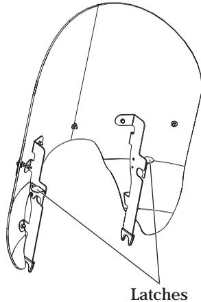
**WARNING!** *Improper windshield installation can result in loss of control, accident and driving hazards for other motorists (if windshield falls from the motorcycle). Always make sure the windshield is fully seated before engaging latches.*
