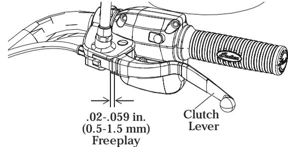
4. Verify that the safety switch activates properly. The engine should not start in gear with the clutch lever released.
