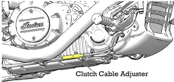
2. While holding the cable, turn the cable adjuster inward or outward until clutch lever freeplay is 0.5-1.5 mm.
