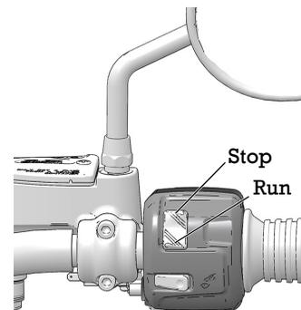
**Tip:** The headlights and any accessories plugged into power ports will remain on until the ignition key is turned off.
