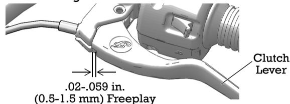
2. Freeplay (gap) is the amount of lever movement from the rest position to the point of cable resistance. Clutch lever freeplay should be 0.5-1.5 mm. Measure the gap between the clutch lever and the lever housing. See page 75. Adjust clutch lever freeplay if necessary.
