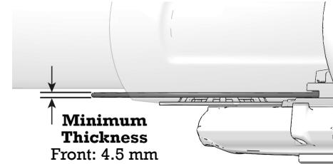
2. Clean discs if minor squeaks develop due to dirt or dust. Apply brake cleaner to a clean shop towel and wipe the discs. DO NOT allow brake cleaner to contact painted or plastic parts. Read all precautions on the label.
