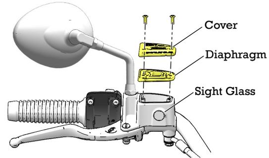
4. The fluid level should be above the minimum indicator mark in the sight glass. Add brake fluid as needed. *Do not overfill.*
