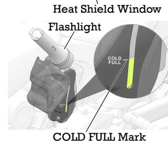
**Tip:** The recovery bottle is vented to prevent overfilling. Coolant will vent onto the ground if overfilled.
