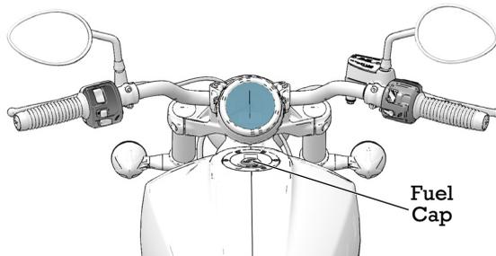
2. Insert the fuel nozzle into the fuel tank filler neck.
