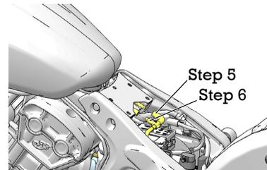
6. Gently pull the straight rubber coupler free of the tube to disconnect the fuel cap recess drain line.
