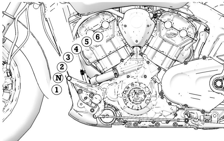
Press downward on the toe lever to shift to a lower gear. Lift upward on the toe lever to shift to a higher gear. Release the clutch lever after each gear shift.
