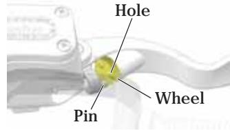
Front brake lever reach (distance to the hand grip) is adjustable.
