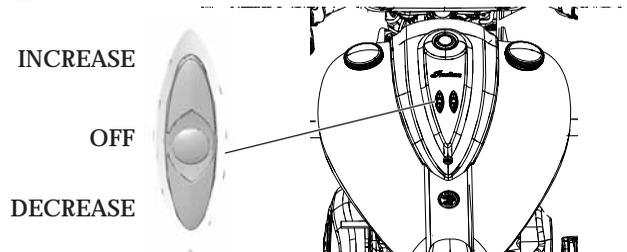
The heaters have 10 heat levels, ranging from OFF (level 0) to highest heat (level 10). Press and release the top of the switch to increase the heat level by one increment. Press and release the bottom of the switch to decrease heat by one increment.
