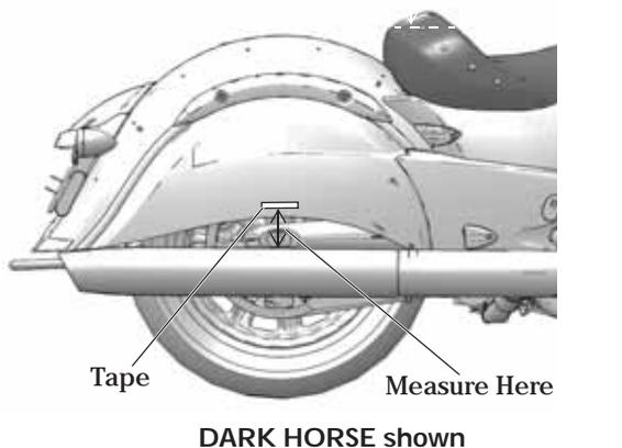
5. Using a suitable lift, raise the motorcycle until the rear shock is completely extended.
