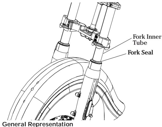
2. Clean the fork tubes to remove bugs, tar or buildup which may cause seal wear or leakage. Inspect the outer surfaces of the inner fork tubes for scratches or damage from foreign objects.
