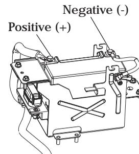
4. Remove the negative (-) battery cable from the battery terminal. Position the cable well clear of the terminal.
