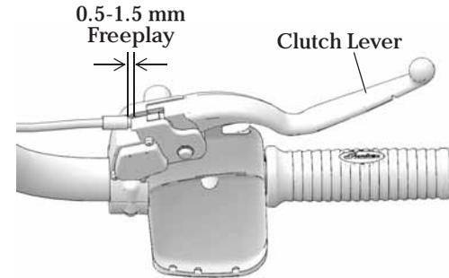
4. While holding the cable, tighten the adjuster lock nut securely.
