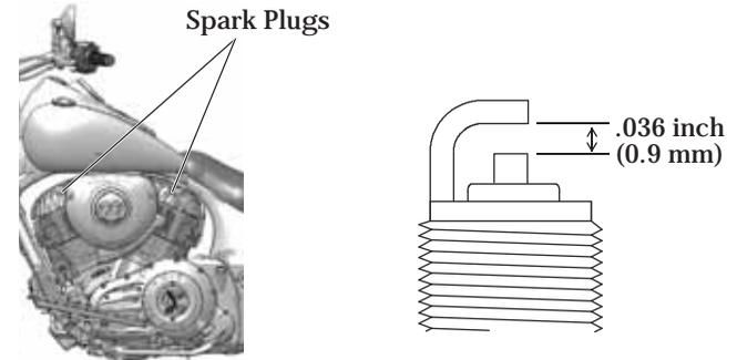
4. To prevent debris from entering the spark plug holes, use compressed air to clean the area around the plugs before removing them.
