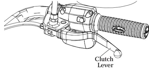
2. Freeplay (gap) is the amount of lever movement from the rest position to the point of cable resistance. Clutch lever freeplay should be 0.5-1.5 mm. Measure the gap between the clutch lever and the lever housing. See page 105. Adjust clutch lever freeplay if necessary.
