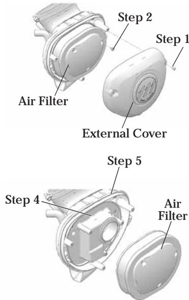
6. Position the air filter assembly against the air box backing plate.
