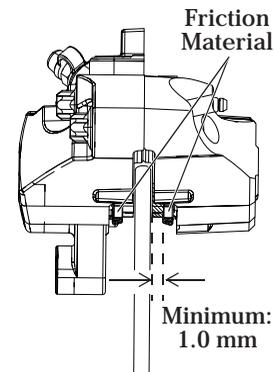
When checking brake pad friction material thickness, check each brake caliper for dampness or stains from leaking or dried brake fluid. If inspection reveals signs of fluid leakage, do not operate the vehicle. See your dealer for service.
