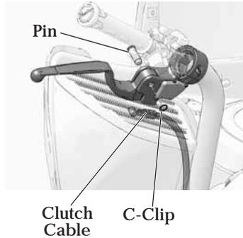
**NOTICE:** During installation of the lever, be aware of the internal clutch switch. Improper assembly can cause damage to the switch.
