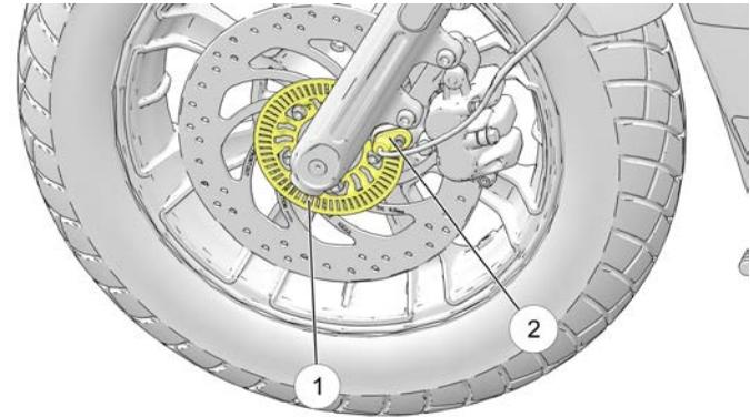
2. Inspect for debris adhering to the end of the wheel speed sensors ②. If contamination is observed, or if you are unable to visually inspect, slide a thin towel across the face of the sensor between the sensor and the tone ring to remove any potential debris.
