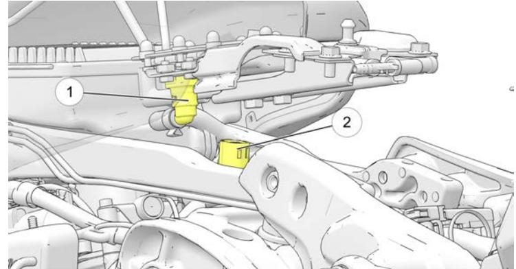
7. Connect the fuel pump harness electrical connector ②. Make sure you hear a click to indicate proper engagement.
