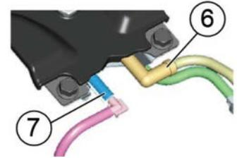
6. Gently pull the straight rubber coupler free of the tube to disconnect the fuel cap recess drain line ⑤ (California and International models ⑦).
