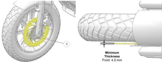
2. Clean discs if minor squeaks develop due to dirt or dust. Apply brake cleaner to a clean shop towel and wipe the discs. **DO NOT** allow brake cleaner to contact painted or plastic parts. Read all precautions on the label.
