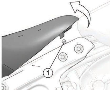
2. Lift the seat to disengage the seat base from the rear frame.
