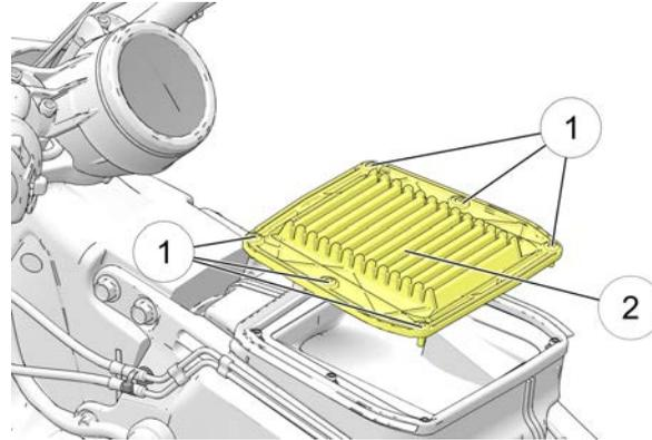
4. Inspect the air filter. Do not attempt to clean the air filter. Replace a soiled or damaged filter with a new filter.
