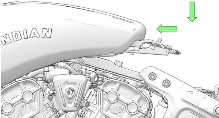
4. Pivot the rear of the tank upward to access the tank bottom. Support the rear of the tank in this position.
