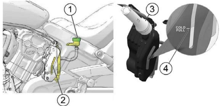
4. Maintain the coolant level at the COLD FULL (4) mark on the recovery bottle (when the fluid is cool).
