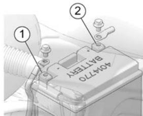
5. Remove the rubber cover from the positive (+) battery cable and remove the cable ② from the terminal. Position the cable well clear of the terminal.
