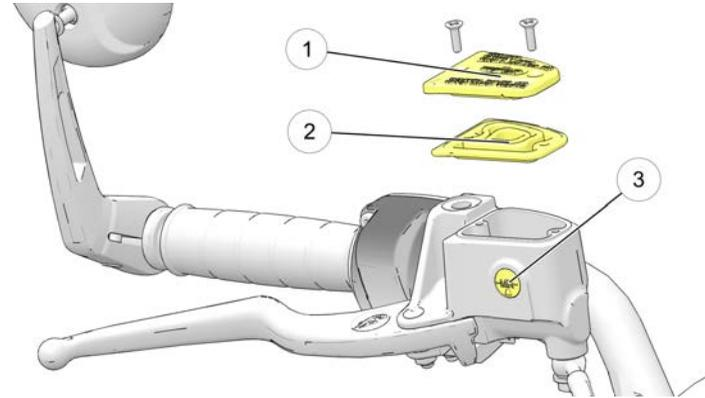
4. The fluid level should be above the minimum indicator mark in the sight glass ③. Add brake fluid as needed. *Do not overfill.*
