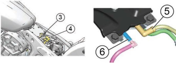
11. Connect the fuel cap recess line ③ (California and International models ⑥).
