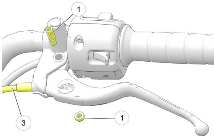
2. Remove any old grease and dirt from the lever and housing. Lubricate the clutch lever and pivot screw with moly assembly grease or all-purpose grease.
