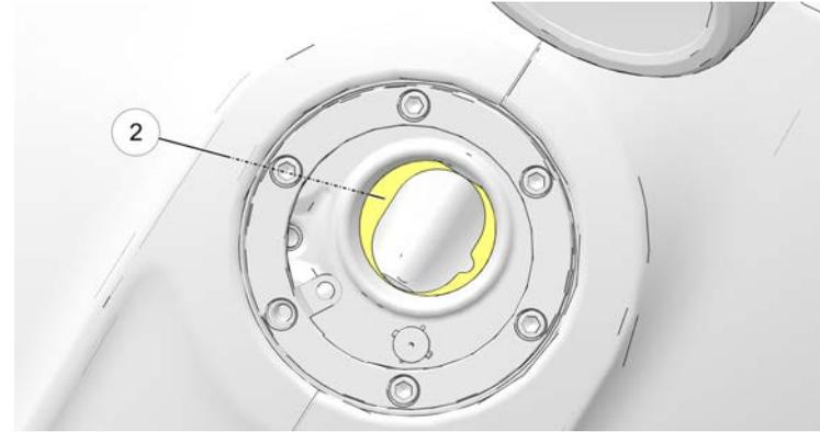
5. Always close and lock the fuel cap before remounting the motorcycle. With the key rotated clockwise, close the fuel cap with your opposite hand and press it down firmly. Turn the key counter-clockwise to secure the lock.
