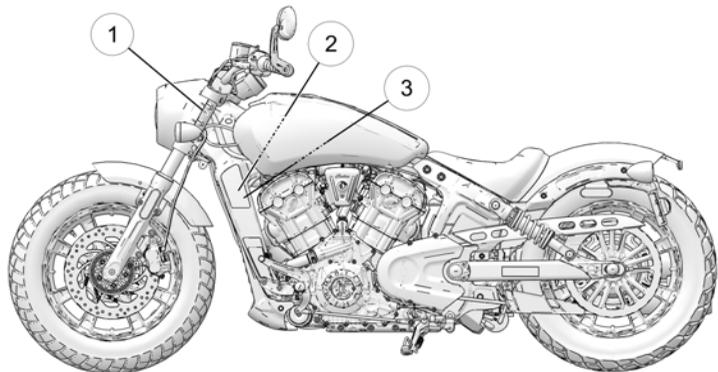
1. Vehicle Identification Number (VIN) (on side of steering head)
