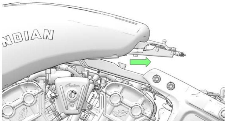
14. Lift the tank up and away from the frame. Reinstall the front isolators if they become dislodged.
