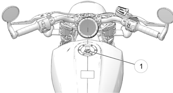
2. Insert the fuel nozzle into the fuel tank filler neck.
